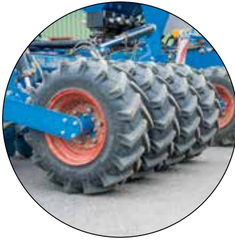
Levelling tines or front tyre packer (optional) for reliable levelling or optimal reconsolidation
